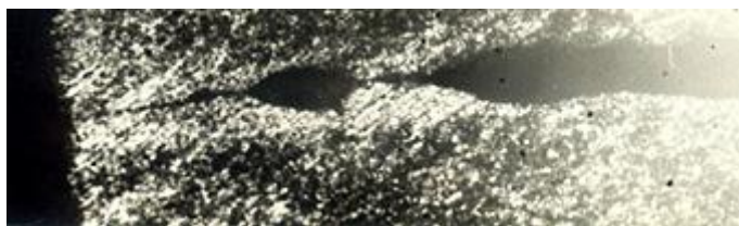
b) 左边环坯裂纹高倍 100x
